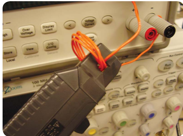
Figure 4-3. Improve the probe sensitivity by winding several turns of the conductor under test around the probe
