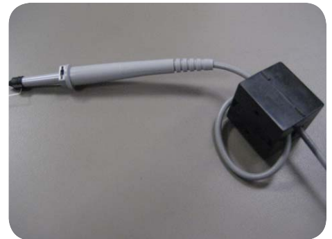
Figure 7-1. Using a ferrite core on the probe cable may help improve probing accuracy
